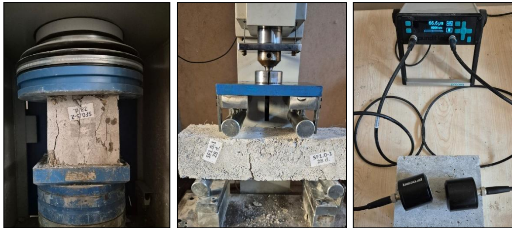
Figure 4. Compressive Strength (a), Flexural Strength (b) and UPV (c)
