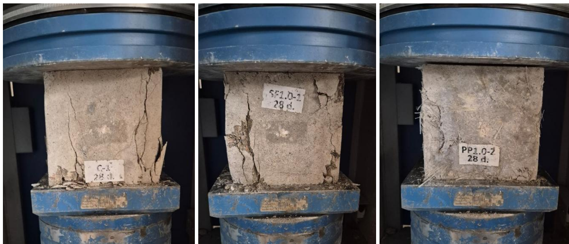
Figure 9. Failure Patterns of RCC Cube Samples
