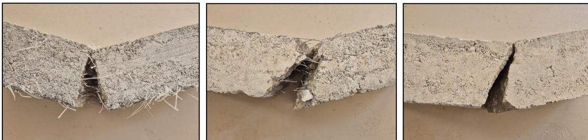
Figure 7. Failure Patterns of RCC Beam Samples
