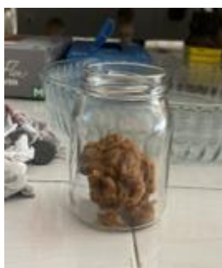
Figure 5. Appearance of the resin formed in Step 1 of Run Order 5 when the glycerol amount was increased.
